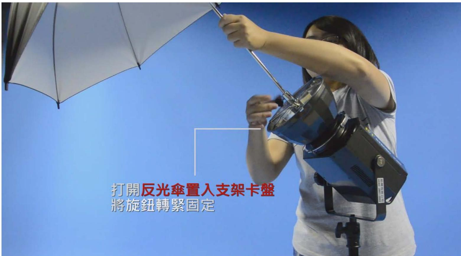
打開**反光傘**置入**支架卡盤**
